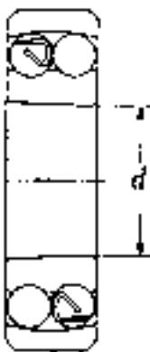
Tapered Bore 13K Taper 1:12
