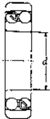
Tapered Bore 12K Taper 1:12
